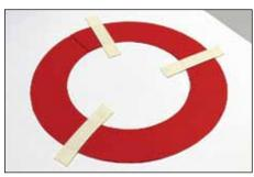
4. Position the overlaps away from bolt-hole locations. As overlaps are made, tape down gasket material to the template on either side of the overlap.
