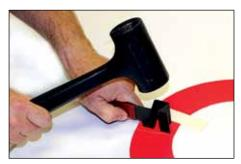
5. Place the Dove-Tail Punch onto each overlap and tap with dead blow hammer to make an initial indentation. Finish the cut by striking the Dove-Tail Punch with solid, flat blows. Top and bottom materials will now have mating dove-tails. Tape the dove-tail joints together for easy handling.
