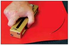
2. From gasket material, cut arcs of material with the proper OD and ID.
