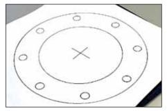
**1.** On a piece of paper or cardboard, lay out the outer diameter (OD), inner diameter (ID) and bolt holes of the desired gasket.
