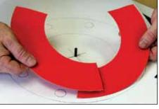
Lay the arcs onto the template, overlapping each end by at least the height of the Dove-Tail Punch to be used.
